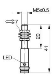
**Inductive Sensors** BES 516-3006-E5-C-S49 M5x0.5 x 41 normally-open Sn=0,8mm shielded
